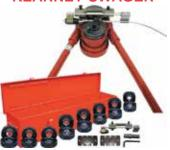
This portable, hand-operated roll type swaging machine will swage MS type terminals onto galvanized and stainless steel cables from 1/16" diameter up to and including 3/16" diameter. Includes machine, a full set of roll dies, terminal gauges and feed guide adapters & instructions in a steel carrying case. Wt. 95 lbs. New manufacture. All replacement parts available.
