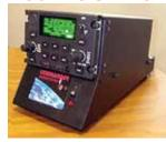
The Commander 2900K is Lone Star Aviation's Docking Station for BENDIX/KING/HONEYWELL KLN 900 DZUS-Mounted GPS. The portable docking station is designed to let you explore the KLN 900 features in a non-flying environment...in the comfort of your home or office. Operation is simple and idea, jeec and Commander's Tray and you are ready to go.
