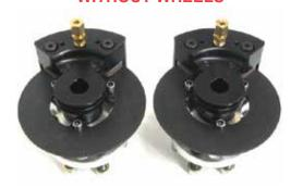
Kit comes complete with two sets of hubs, 4.5" rotors, calipers, brake pads as shown along with two 8" axles with hardware, 15 feet of high pressure brake line and one bleeder kit. 5/8" or 3/4" bearing options. 5/8 Bearing ......P/N 15-05703 3/4 Bearing .......P/N 15-08293
