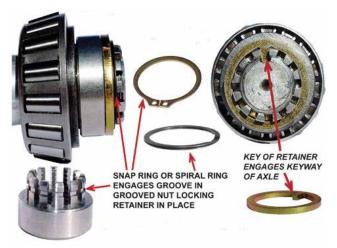
True-Lock aviation fastener systems reduce premature wear on your wheel-end assembly parts (brakes, bearings, axles, including tires and wheels). The True-Lock system eliminates the conventional axle nut system's inherent inferior torque setting characteristics imposed by the castle nut and cotter pin (end-play).
