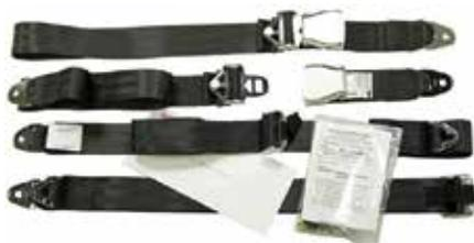
FAA approved STC / PMA kit for the installation of 3 Point Diagonal (Single Strap Over) fixed strap (manually adjustable) shoulder harnesses in the 2 front seats (pilot and co-pilot) of an aircraft that did not come with factory installed shoulder harnesses.
