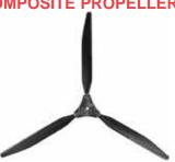
Warp Drive's Advanced Composite Carbon Fiber propeller has a structural strength near that of metal propellers. Because of the stiffness achieved by using carbon fibers, the prop will do very little coning (bending forward) under power. Proper fiber placement allows the prop to flex torsionally for maximum cruise efficiency. The strongly fixed position of the blades along with optimum torsional performance translates into more thrust than conventional propellers.
