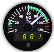
Electronics International Inc. will configure the TR-1-NG to the range limits provided by the pilot/owner and/or mechanic. The data provided must match your aircraft's POH/AFM and all changes required by AD's, Supplements and/or STC's. Also, limits may be crosschecked against the instrument previously mounted in the aircraft panel. If any of the information provided on this form is incorrect and requires a reconfiguration, there will be an additional fee.
