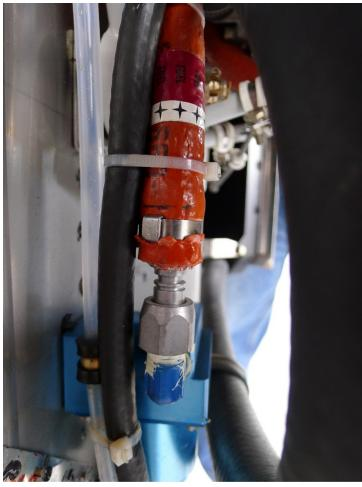
Stock System 2 (Combination Rubber and Teflon) – Rotax changed over their fuel system to Teflon carb lines at some point. These are integral firesleeve Stratoflex 101-4 orange fuel lines. These lines were combined with rubber lines on the rest of the fuel system. The arrow points to the Carb line. In higher corrosion environments, the collars may corrode as they are not stainless steel and the hose does not utilize a silicone sealing cuff on the end.
