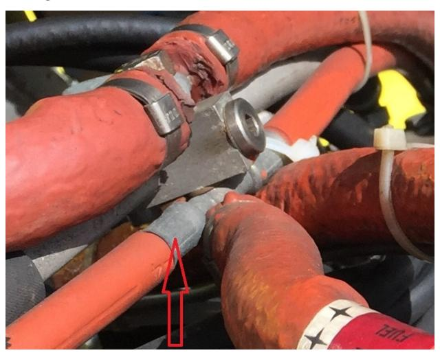
Stock System 3 – All Teflon Fuel System - The newer RV-12 kits are shipping with an all Teflon Fuel System. It appears that most of the hoses are Conductive Teflon. The only hose that is Non-Conductive Teflon is the VA-216 Hose assembly. There is no longer a recommended replacement schedule on these hoses, except for the VA-216 which has a 10 year recommended replacement schedule per the Van's manual.
