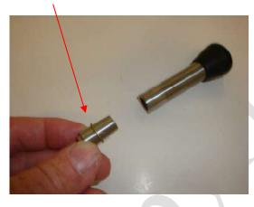
**T98-1** - Installation of CLoc® or Camloc® 2000 Series Retainers (2600-LW and 27S5-1). Place retainer onto base of stud (cup); simply press retainer until seated.
