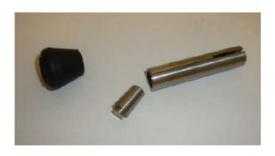
T26 - Installation of CLoc® or Camloc® R4G Snap Ring Retainers – Remove cap and taper insert.
