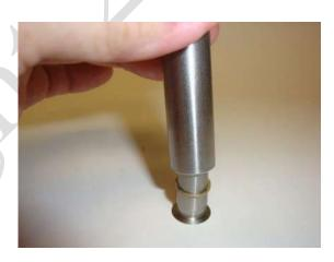
Push R4G Retainer onto grommet (Install grommets-retainers then install studs with 4P3 Pliers).
