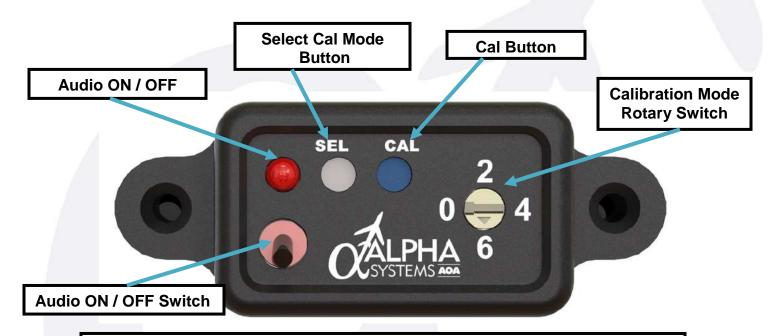
The Falcon AOA system requires a remote switch panel that must be mounted in a location near the pilot for activation of the calibration procedures and turning the audio ON and OFF. It can be anywhere within the cabin and comes with a 6 foot extension cable.
