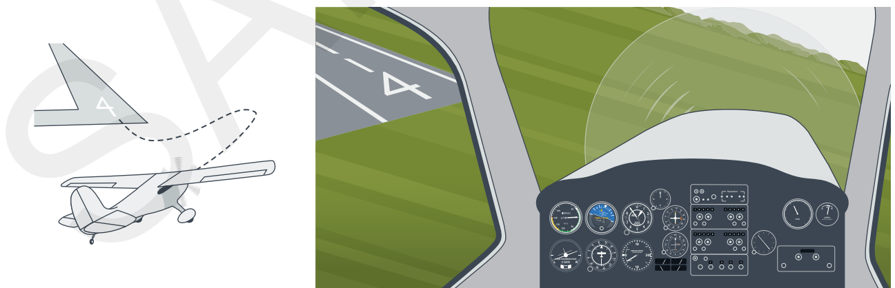
Fig. 14-1. Pilot sees that the plane will fly past the runway if the rate of turn is not increased.
