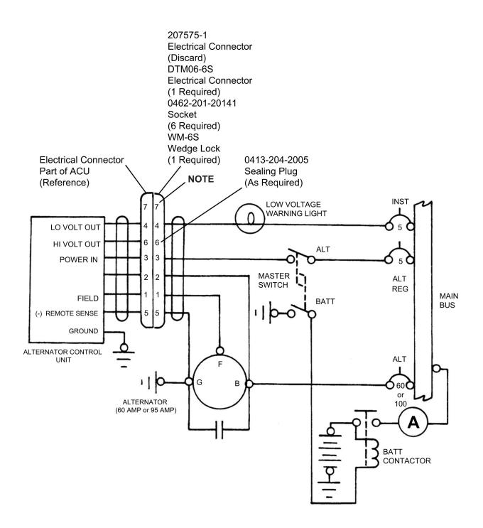
**NOTE:** Pin 7 of discarded ACU and discarded ship-side connector are unused. New ACU and ship-side connector only have 6 pins.
