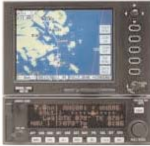
A powerful MFD, the KMD 150 adds color and enhanced situational awareness to existing GPS installations.
