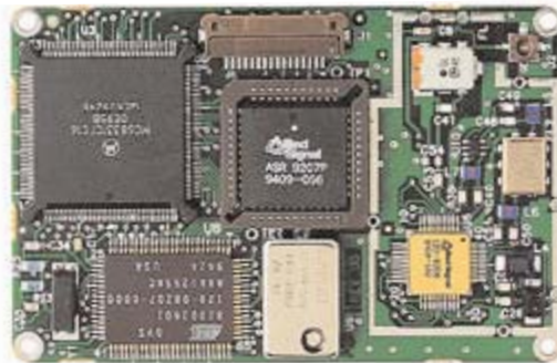
Able to simultaneously track up to eight satellites, the KLN 90B's parallel GPS receiver was designed for compatibility with most existing avionics. A marvel of compactness, this GPS engine (shown full size) enhances both reliability and performance.
